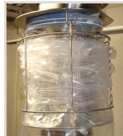
Continuous Liner System
